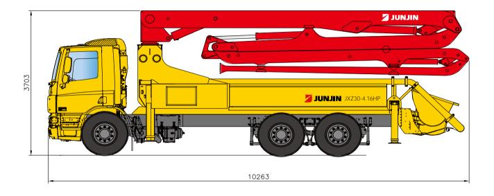
\* Remark : Standard specification with DAF 6X4. Dimension depends on truck specification.
