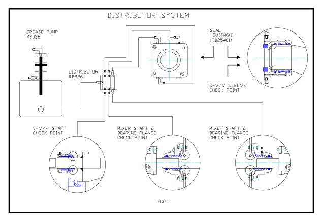
Automatic greasing system does not work if one of the lines is blocked.
