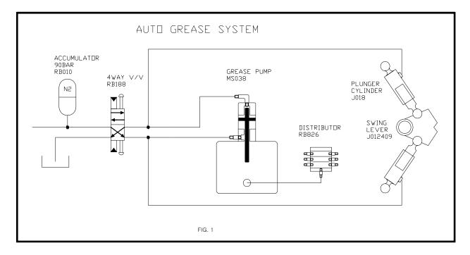
P-line of accumulator pressure is supplied to the grease pump, and grease is supplied to the each component through the distributor.
