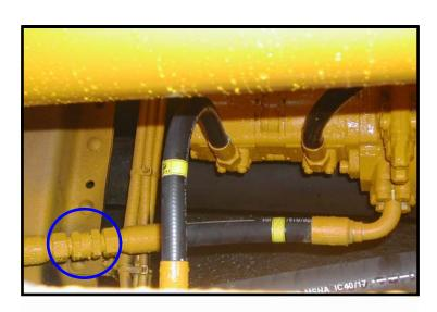
Fig. 21 Line check valve
