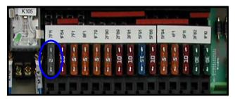
Fig. 3 Removal of fuse(7F11, 2A) for safety
