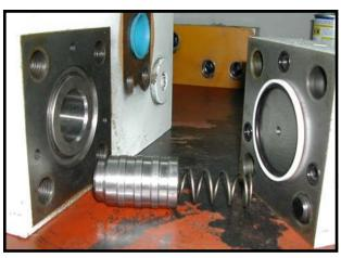
Fig. 7-1 Logic element
