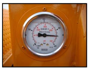
Fig. 5 Main pump pressure gauge
