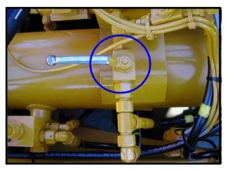
Fig. 1 Manual shut-off valve for accumulator pressure drain
