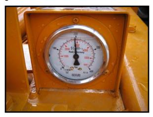
Fig. 22 Pressure gauge for accumulator pump
