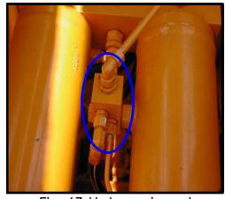
Fig. 17 Hyd. sensing valve (Pistin side)
