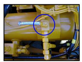
Fig. 25 Shut-off valve for accumulator pressure drain
