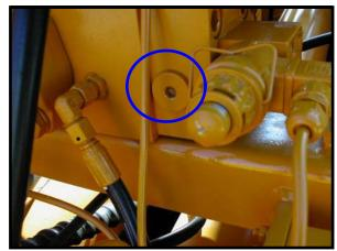
Fig. 6 Shuttle valve next to the solenoid valve
