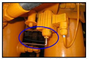
Fig. 1 Volume control reducing valve and manual volume control with allen wrench
