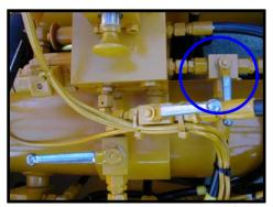
Fig. 2 Shut-off v/v for max. output(Rexroth A11V260, A20V190)
