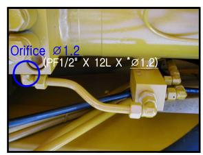
Fig. 16 Hyd. sensing valve (Rod side)
