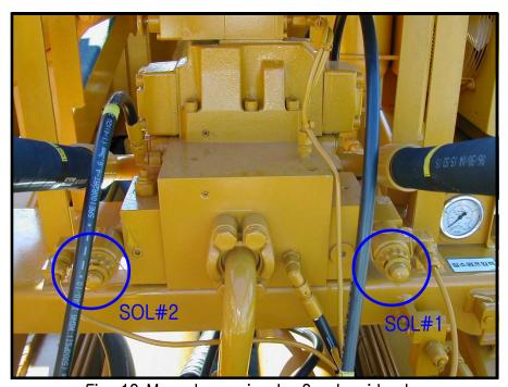
Fig. 12 Manual pumping by 2 solenoid valves
